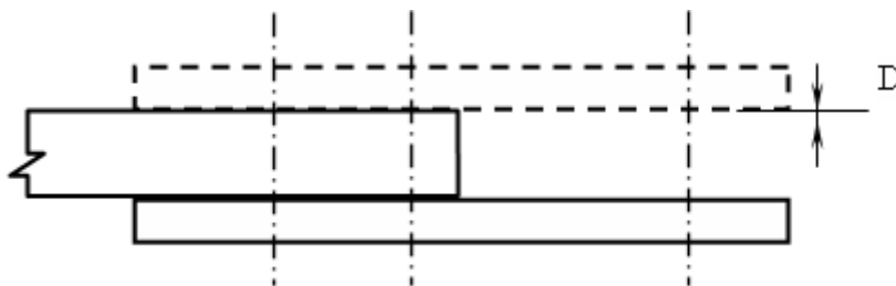
Figure 3 — Difference of thickness between components of a common ply
